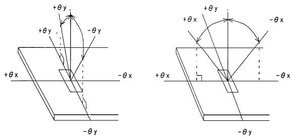
Fig. 4 Definition of Viewing Angle
