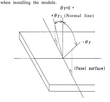
Fig. 12 Dot matrix LCD viewing angle
