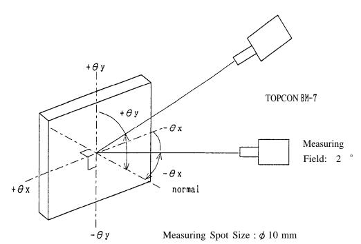
8x: Angle from "normal" to viewing surface rotated about the horizontal axis.
